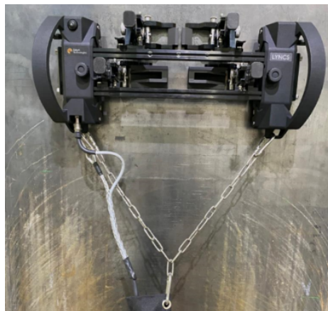
Figure 17: Strain relief chain for the cable management
