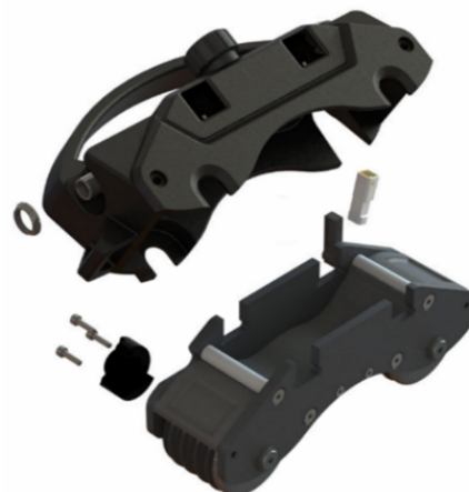
Figure 39: Encoder replacement step 4
